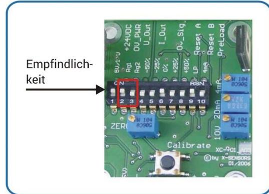
The fine adjustment of the full scale can be made with a potentiometer. For this purpose, compare the full scale value simulated by means of a strain gauge simulator. By turning the potentiometer, you can set the full scale value to the desired value.
