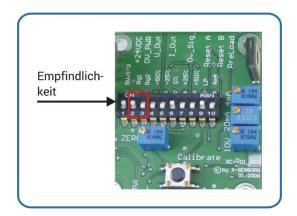
The fine adjustment of the full scale can be made with a potentiometer. For this purpose, compare the full scale value simulated by means of a strain gauge simulator. By turning the potentiometer, you can set the full scale value to the desired value.
